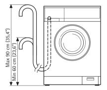
The upright standpipe should have a minimum, length of 30 cm (12") from the bottom of the elbow to the top of the pipe (see diagram). Make sure that it is designed in such a way that the end of the drain hose cannot be covered with water. Longer drain hoses are available in lengths of 2.7 and 4 metres from your AEG Service Force Centre.
